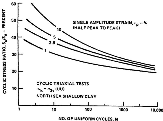
Fig. 3. Effect of cyclic storm loading on clay soil (after Lee and Focht, 1976b).
