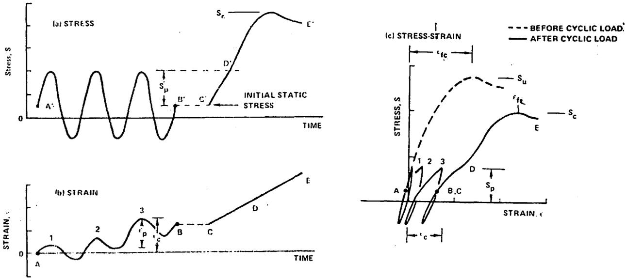
Fig. 1. Illustrative cyclic-static test record. AB and A'B' equal the cyclic stress-strain path; BC and B'C' equal the rest and adjustment period following cyclic loading; CDE and C'D'E' equal the one-directional static loading test; and the dashed curve refers to one directional static loading test on an identical sample with no previous cyclic loading (after Lee and Focht, 1976b).
