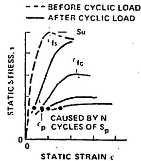
Fig. 2. Illustration of static strength after cyclic loading (after Lee and Focht, 1976b).
