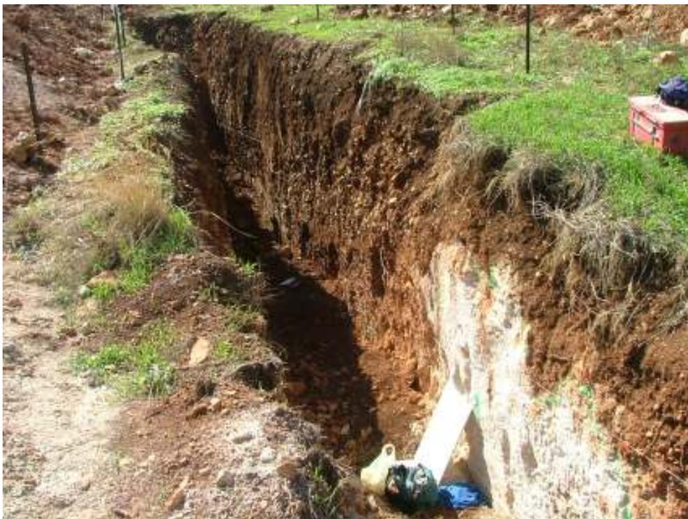
***Fig. 8 – The transition zone (White color – Adulam Formation; Brown color – colluvial and alluvial sediments)***
