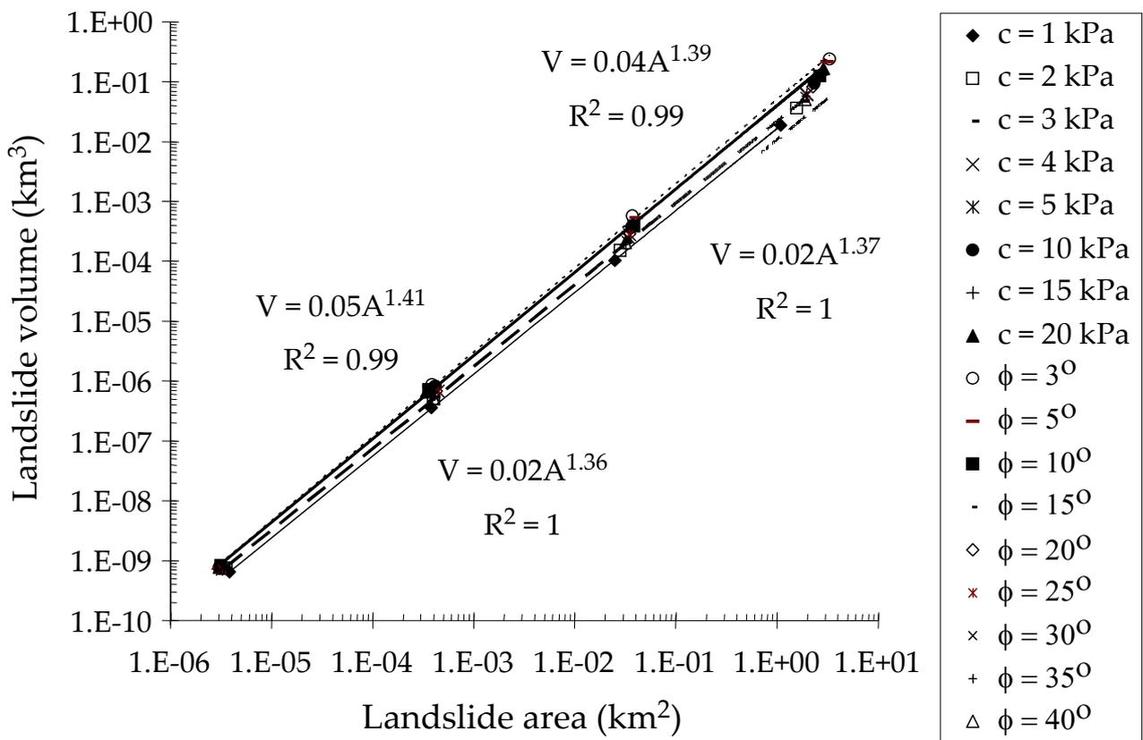
Figure 5 .Model predicted area (A) vs. volume (V) of landslides at fixed unit weight ( $\gamma = 18\text{kN/m}^3$ ), fixed slope angle ( $\beta = 26.57^\circ$ ) and changing slope height (H = 1, 10, 100, 1000m). Shown here are the trend lines and regression equations of the 4 extreme cases: (a) c = 1kPa ,  $\phi = 25^\circ$  (thin solid line); (b) c = 20kPa ,  $\phi = 25^\circ$  (heavy solid line); (c) c = 5kPa ,  $\phi = 3^\circ$  (dotted line); (d) c = 5kPa ,  $\phi = 40^\circ$  (dashed line).
