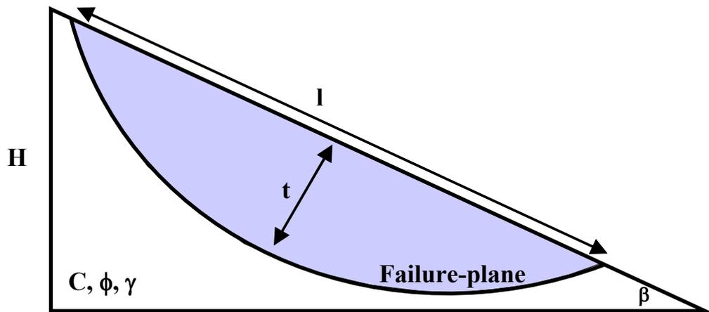
Figure 2. 2D schematic cross section of a landslide (of thickness  $t$  and surface length  $l$ ), originating from a slope of height  $H$  and slope angle  $\beta$ . This is the configuration used in our model .
