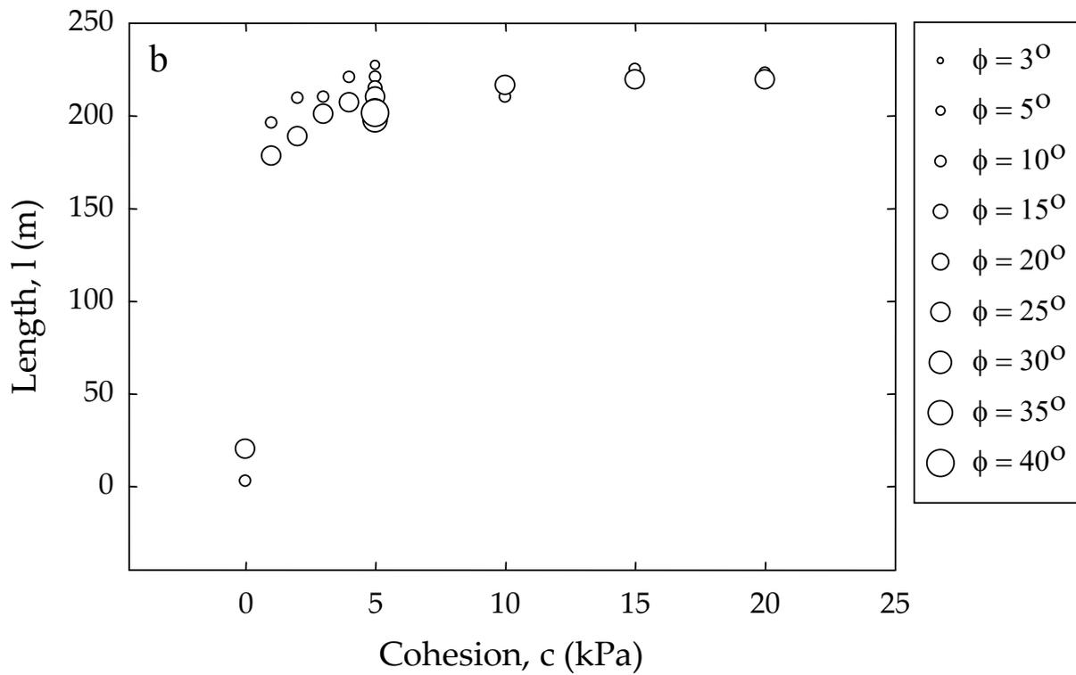
Figure 3. Model predicted landslide geometry (thickness and length) as a function of mechanical properties (cohesion and angle of internal friction). The slope height,  $H$ , is 100 m and unit weight,  $\gamma$ , is 18 kN/m<sup>3</sup>. (a) landslide thickness,  $t$ ; (b) landslide length,  $l$ .
